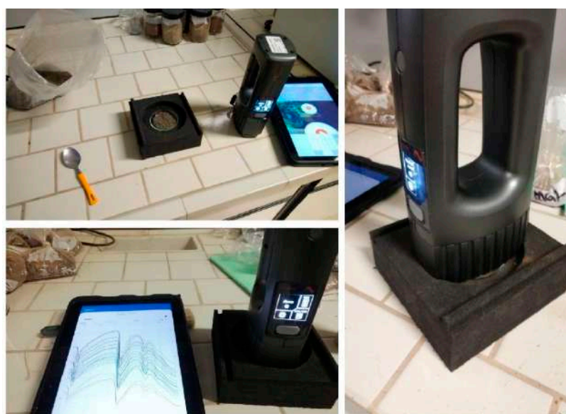
Figure 2. The spectral measurements carried out by Neospectra Scanner. All the measurements were visualized and recorded in the dedicated Android tablet, connected by bluetooth signal.
